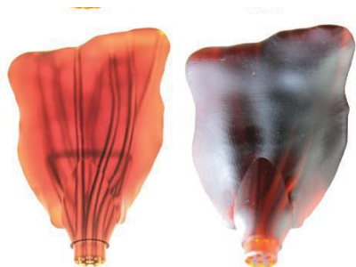
Photos of 3D printed applicators, with and without LED backlights.
